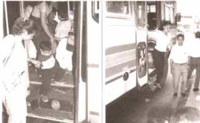
Figure 7. Very small size of step track represents a greater risk of accident when descending.
